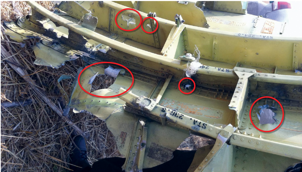
Figure 9: Part of the inside cockpit roof, indicating penetration with objects from outside. (Source: DCA)
