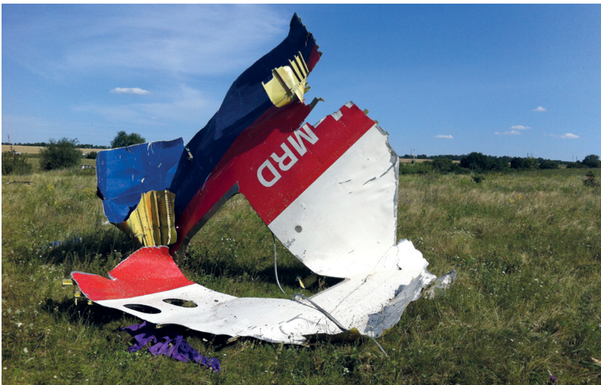
Figure 13: Aft fuselage skin, right side, with partial registration of the aircraft. (Source: NBAAI)
